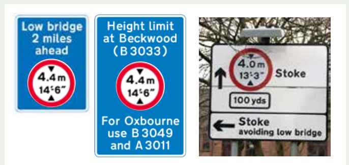
Figure 13: Advance warning signs
